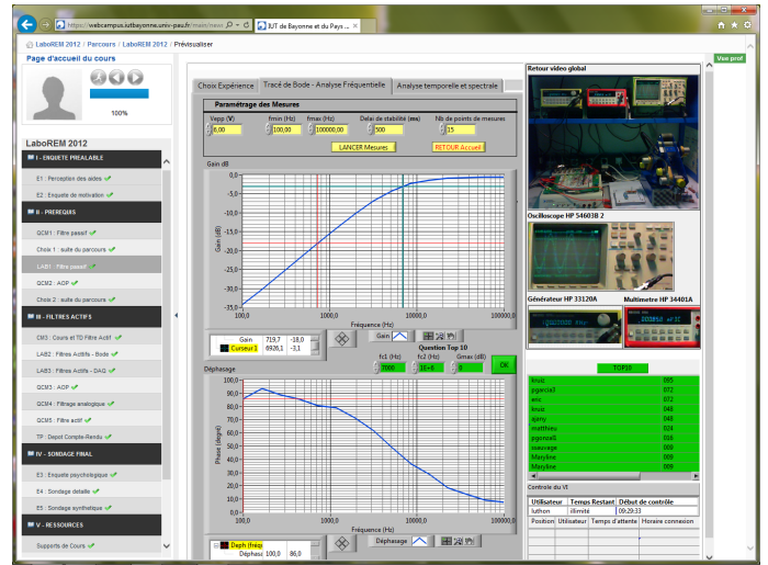
Figure 5. Client rich interface showing a remote front panel: left) learning steps of the pedagogical scenario; center) experimental results (Bode plots of a high-pass filter); right) video feedback of lab and instruments, Top 10 list and queuing list of users.
