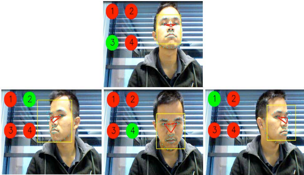
Figure 6 - Different state detection. The state is indicated by the number of the green circle. In state1 the student looks left; in state 2 he looks right; in state 3 he looks up; and in state 4 he is concentrated on the given task.
