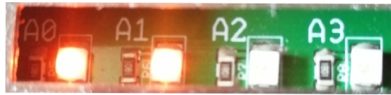
Fig. 13. 4 LEDs on the motherboard indicate the selected plug.
