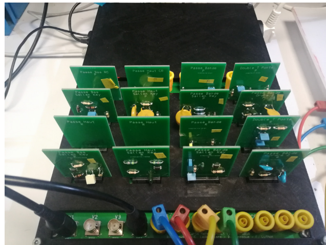
Fig. 17. BNC, bananas and plugs connected to the Laborem Box.
