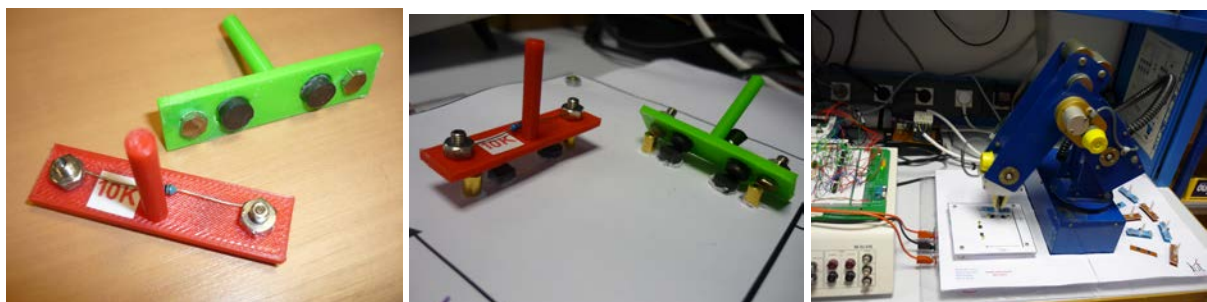
Figure 6 – a) Components equipped with magnets; b) Robot placing a component on the board.
