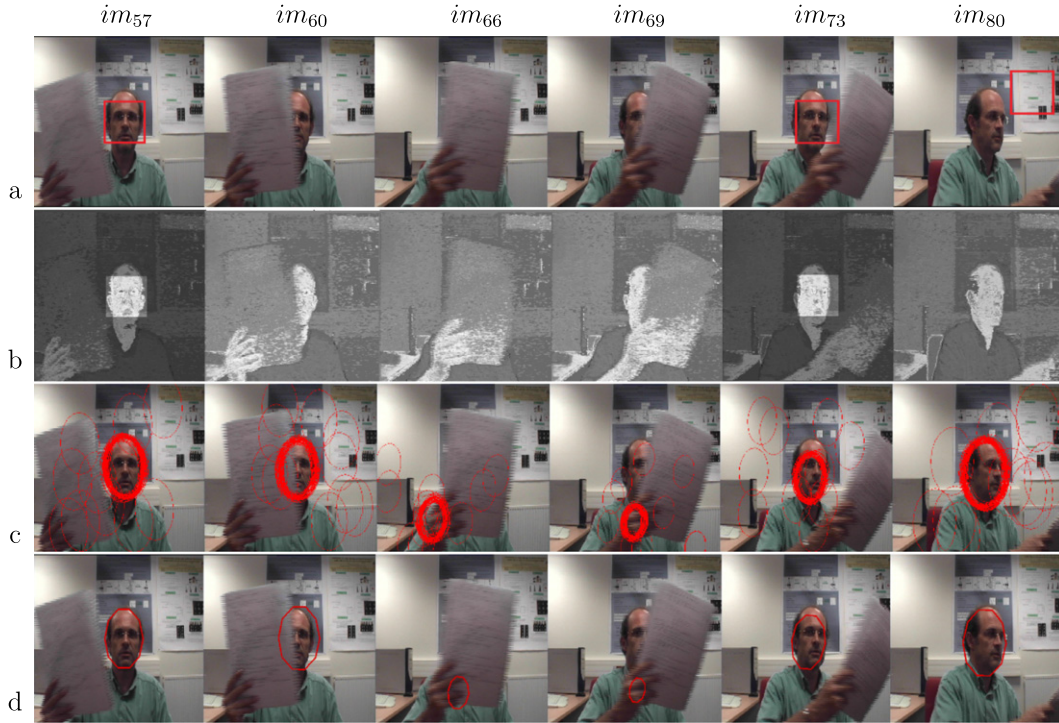
Fig. 12. Face tracking for sequence #1: (a) Bounding box (in red) supplied by the VJ face detector; (b) Pignistic probability stemming from the face model; (c) Particle filter particles during the centre estimation step of X_t ; (d) Ellipse resulting from particle filter.
