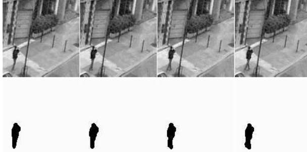
Figure 2: Top) Street sequence with a moving pedestrian; Bottom) Masks of the moving body detected after relaxation (black = moving label, white = static label).
