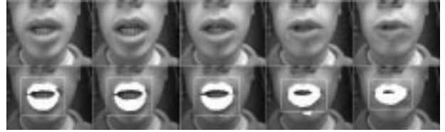
Figure 7: Top: sequence of luminance images ;Bottom: sequence of final lip hue fields with ROI superposed on the luminance.
