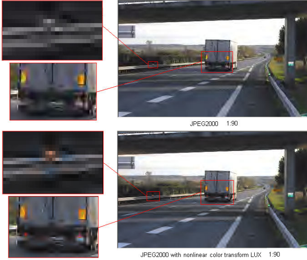
Fig. 5. Compression with JPEG2000 (ratio 1:90 ; Dwt9/7): comparison between YCrCb (top) and LUX (bottom)
